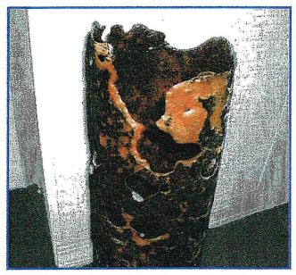
Figure 5. Corroded well casing.
