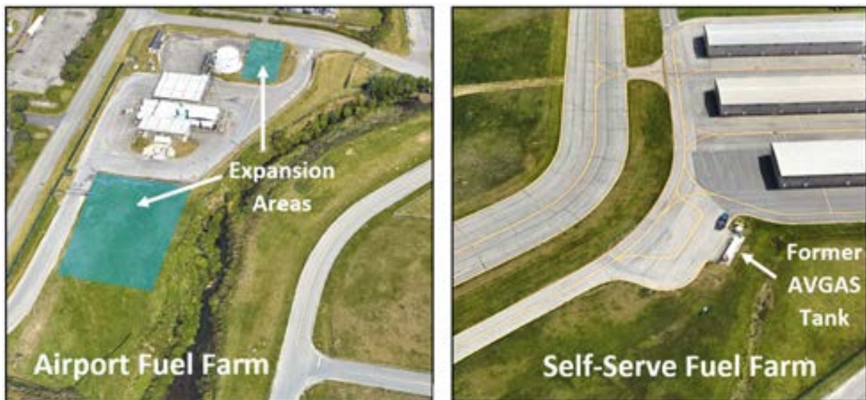
Figure 5-23 – Existing Aircraft Fuel Farms and Expansion Potential
