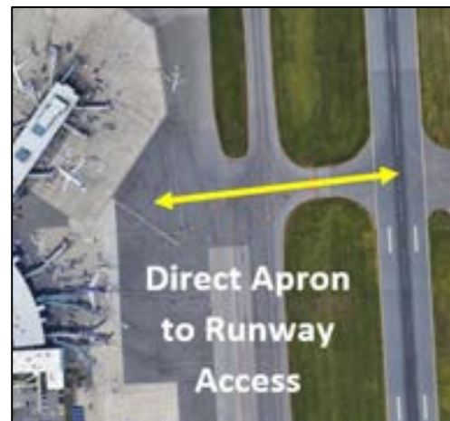
Figure 4-10 – Direct Apron-to-Runway Access
